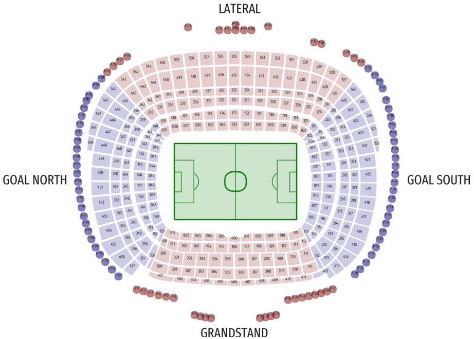
Fig. 1 Camp Nou stadium schema Gates are represented as circles, with their respective names in black (as P-# of gate). The other polygons represent the different inlets of the Camp Nou as numbers, where the first number always indicates the floor of the inlet, ranging from 0 to 5. The colors in the inlets or sections represent the main sections of the stadium (bottom seats in red of the plot are the grandstand, right and left seats in blue show the goal south and goal north sections of the stadium respectively, and the top seats in red show the other lateral section)
