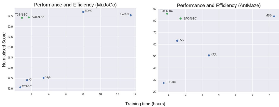
Fig. 7 Performance and efficiency. Average training time and normalised score across MuJoCo and AntMaze tasks. TD3-BC-N and SAC-BC-N can match the performance of ensemble-based approaches while retaining the computational efficiency of those based on behavioural cloning
