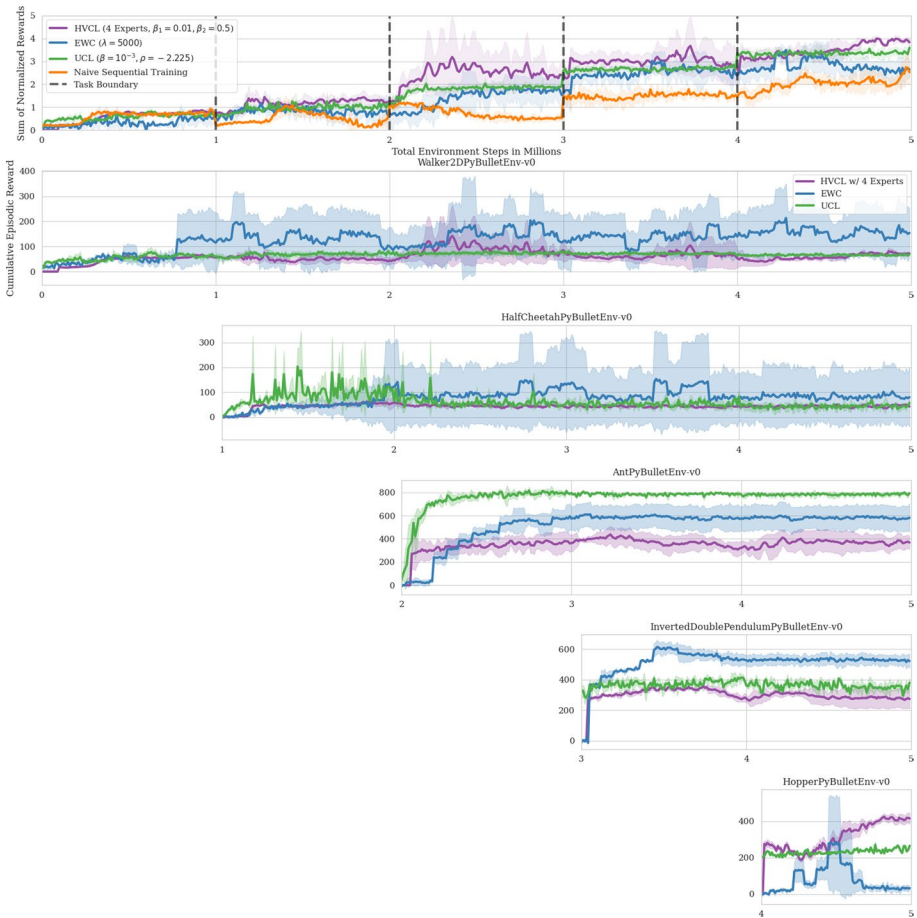
Fig. 5 Continual reinforcement learning. The upper row shows the cumulative normalized rewards over time across the five reinforcement learning tasks. Each vertical dotted line indicates a change in environment after 1 million frames. Performance is computed according to Eq. (16) after each frame and thus represents the total reward achieved by the agent summed over t tasks (with a maximum normalized reward of one per task). Thus, a value close to t indicates no forgetting, while 1.0 shows the total forgetting of old tasks. The lower row shows the absolute cumulative episodic reward in each of the five environments given pre-training on the preceding tasks. We compare against EWC (Kirkpatrick et al., 2017) and UCL (Ahn et al., 2019). The lower bound is given by a naively trained dense neural network using SAC (Haarnoja et al., 2018) without CL and without access to old environments
