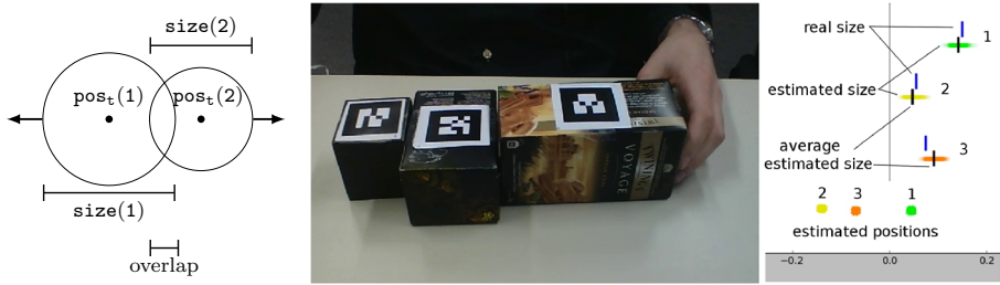
Fig. 14 Learnsize scenario. Sketch on the left : the objects are pushed away from each other when they overlap, applying a displacement. Picture on the center with 3 objects. The right figure represents the estimated objects’ positions (yellow, orange and grey), and the estimated size (one point per sample) using artificial dynamics. The blue lines are the real size and the black lines the average estimated size. The distance is measured in meters
