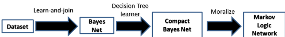
Fig. 1 System architecture for context-sensitive moralization: learning a compact Markov logic network from an input relational database
