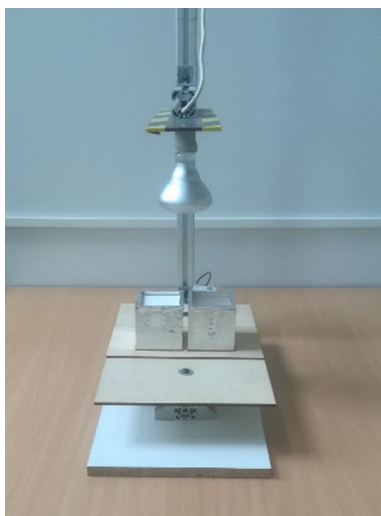
Fig. 1 The arrangement of laboratory-scaled “sun test”
