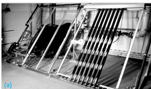
Fig. 6 Photographic presentation of setup and cross-sections of an ETC with a heat pipe (HP) inside a without PCM, b with PCM [28]
