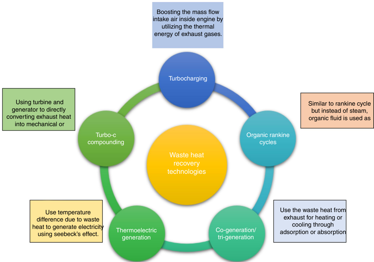
Fig. 11 Waste heat recovery methods
