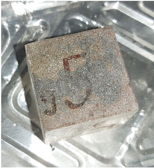
Fig. 6 Boron carbide-containing specimen exposed to 900 °C
