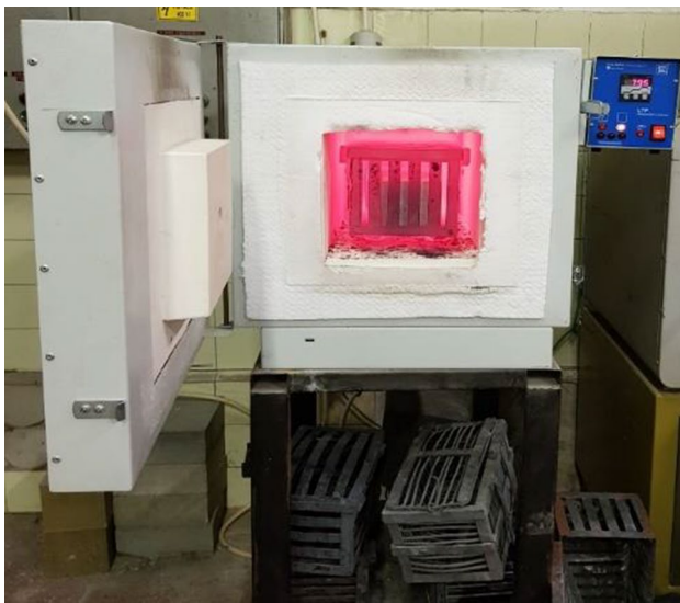
Fig. 4 Electrical furnace containing a steel cage
