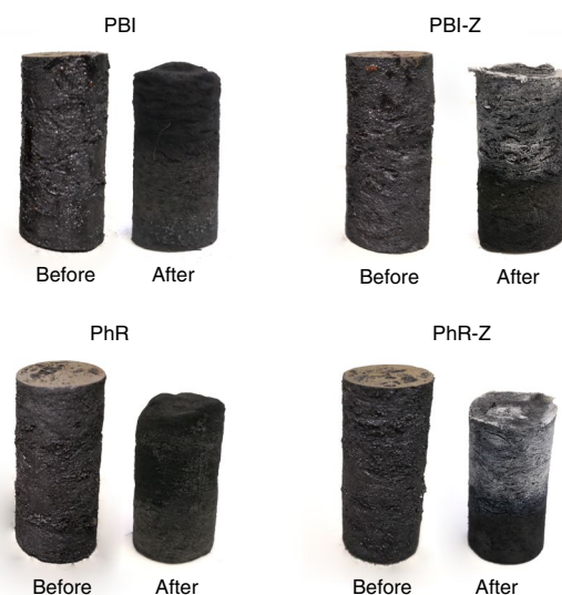
Fig. 9 Ablative material samples after the oxy-acetylene flame exposure
