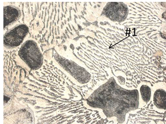
Fig. 2 The microstructure of the Zn–Al alloy, a cooling rate 0.1 \text{ °C s}^{-1} , “fine eutectic” \alpha' and \eta ; #1—eutectic \alpha' + \eta
