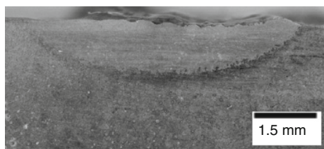
Fig. 2 Cross section of the investigated AlSi 9 Cu 4 surface layer after laser treatment ZrO 2 + TiC, laser power 1.5 kW
