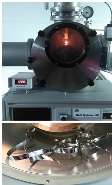
Fig. 1 Bühler melt spinner SC station for making the metallic glasses
