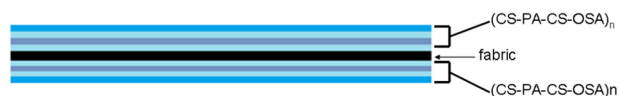
Fig. 3 Arrangement of the nanolayers obtained by the layer-by-layer method in the multilayer coating (based on [26])
