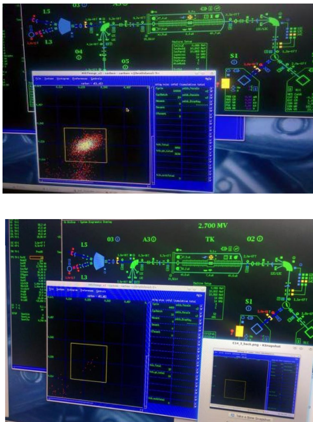
Fig. 7 Two-dimensional ^{14}\text{C} spectrum of the NIST oxalic acid standard (OXA II) (top) and corresponding background (bottom) measured by the end-of-the line ionization chamber
