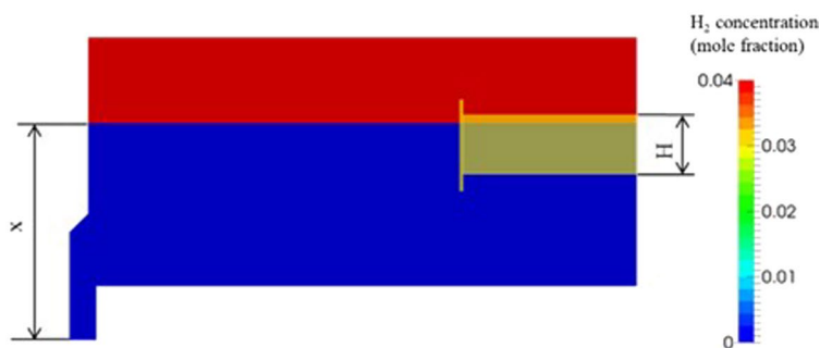
Fig. 3 Hull canister upper model initial conditions (2D axisymmetric model)
