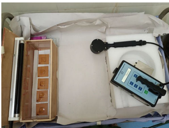
(a) Experimental setup showing UV irradiation chamber & contamination monitor for counting (color)
