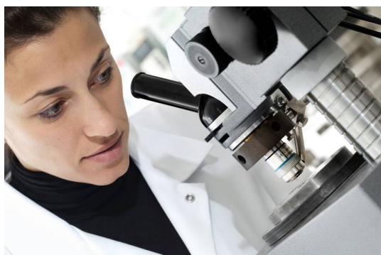
Fig. 4 Dr Maria Marouli optically measuring the source thickness using a vertically traveling microscope with distance probe. It is currently replaced with a 3D-coordinate measuring machine [71]
