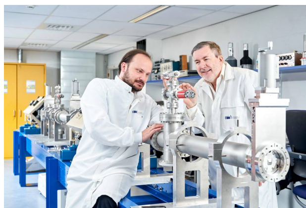
Fig. 12 Drs. Krzysztof Pelczar and Stefaan Pommé at the construction of the A-TOF facility, which measures the energy of alpha particles emitted in radioactive decay. The energy resolution is improved by measuring the time-of-flight of the alpha particles over a flightpath of several meters. The aim is to provide accurate nuclear decay data of alpha-emitting nuclides
