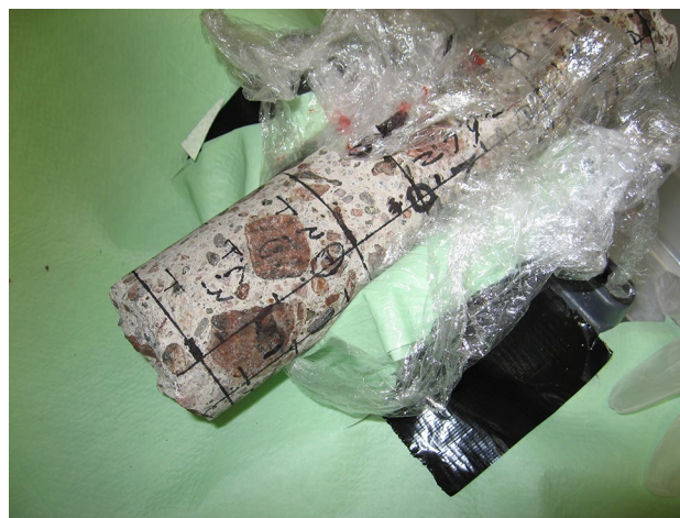
Fig. 1 Picture of the FiR1 biological shield concrete core (diameter 7 cm)
