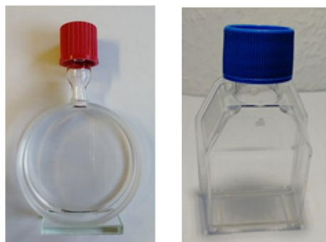
Fig. 2 Flasks for the measurement of decontaminated mercury samples, left: geometry-optimised cylindrical sample flask, right: commercially available cell culture flask
