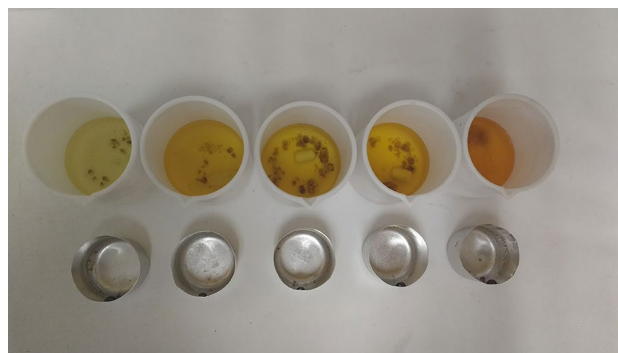
Fig. 2 PTFE beakers and Pt–Au crucibles containing the digested concrete samples (1–5 g left to right) in 5 M \text{HNO}_3 nitric acid
