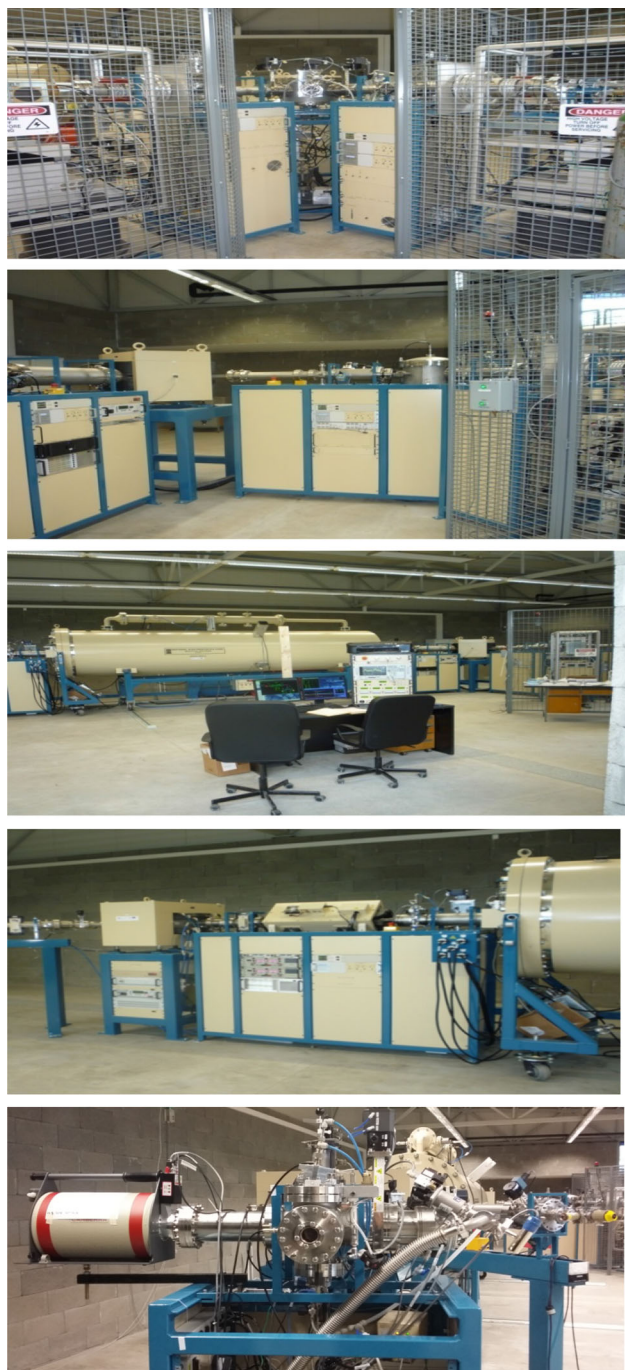
Fig. 19 Tandem accelerator laboratory (from the top: Alphasources and SNICS ion sources, injection line, Pelletron, analyzing line with switching magnet, end of the line PIXE/PIGE chamber)
