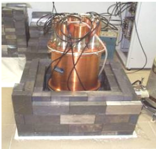
Fig. 6 Construction of the anti-Compton gamma-ray spectrometer in the IAEA-ELs Monaco underground laboratory (100% HPGe detector surrounded by NaI(Tl) detectors in a lead shield)
