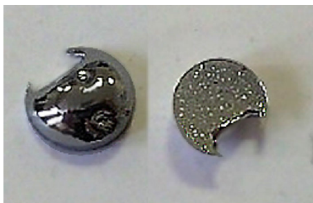
Fig. 3 Partially melted molybdenum pellet made of 1 350 mg of the Mo powder
