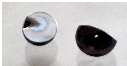
Fig. 4 Molybdenum bead after first pass through the rolling mill set too tightly
