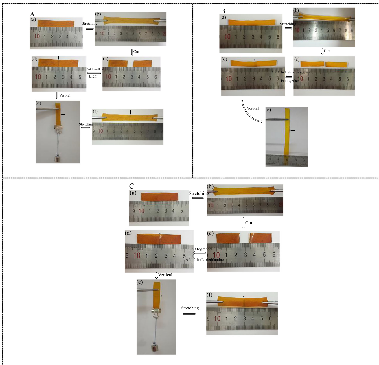
Fig. 12 A Light self – healing processes of IPN hydrogel (Where, (a) is the virgin sample 4.8 cm, (b) is stretched to 9.0 cm of the virgin sample, (c) is cut, (d) is put together, (e) is placed vertically after self-healing, (f) is stretched to 8.2 cm of the self-healing sample, “→” shows the self-healing placement), B Acid self – healing processes of IPN hydrogel (Where, (a) is the virgin sample 5.5 cm, (b) is stretched to 8.6 cm of the virgin sample,
