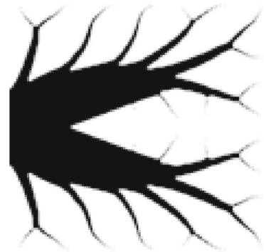
Fig. 19 Resulting smooth topologies of heat conduction problem obtained by non-penalized SEMDOT under different target volume fractions
