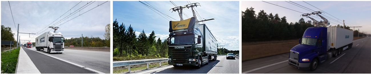
Fig. 1 Examples for test tracks equipped with overhead wiring in Germany (left; source: Siemens AG), Sweden (middle; source: Scania CV AB), and the USA (right; source: Siemens AG)
