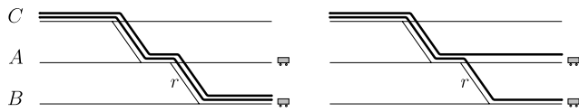
Fig. 3 A BP for the case that station A has a final deficit, and station B has a final surplus: the train length on trip r is decreased
