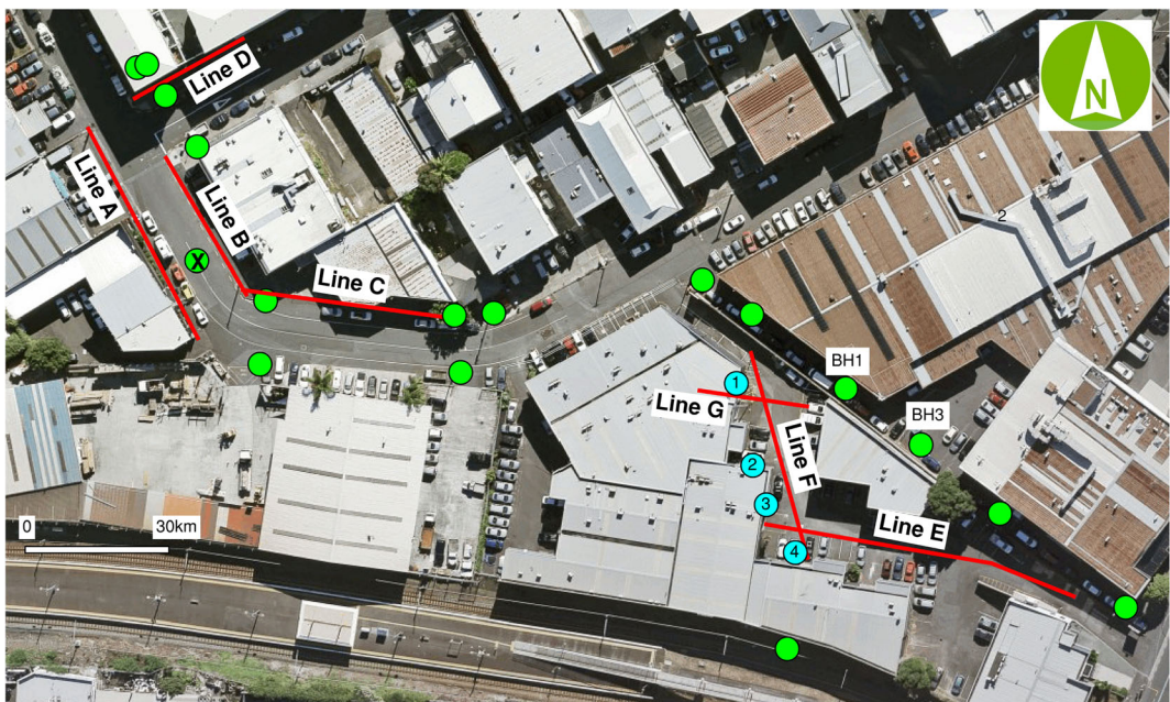
Fig. 7 Locations of the ReMi seismic arrays (red) near Mt Eden Train Station. Green circles show boreholes nearest the seismic survey locations at the time of the investigations. The cyan circles
