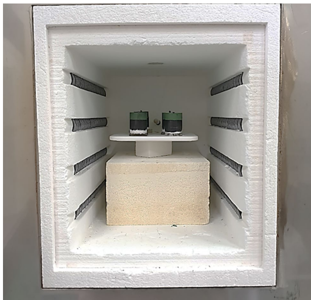
Fig. 7 Demonstration of batch production of (Gd,Y,Er)BCO ternary bulks via IG technique in a small box furnace ( 21 \times 15 \times 16 \text{ cm}^3 )
