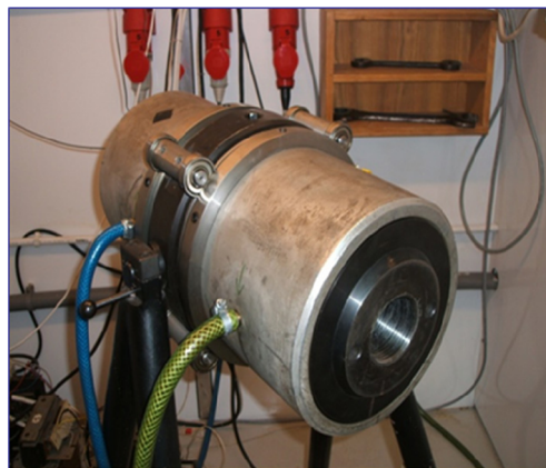
Fig. 1 Pressure chamber. Maximum isostatic pressure of 1.6 GPa and maximum annealing temperature 2000 °C
