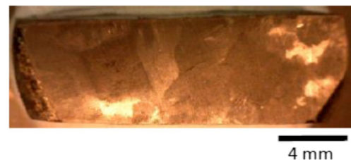
Fig. 5 Photograph of the top surface of the four-seeded YBCO sample after polishing. Growth of only two grains can be clearly seen
