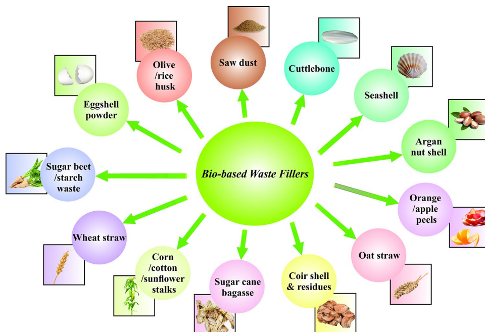
Fig. 1 Common bio-based waste fillers used for the development of biodegradable polymer composites. Amongst various bio-filler resources, widely-used ES exhibits unique properties
