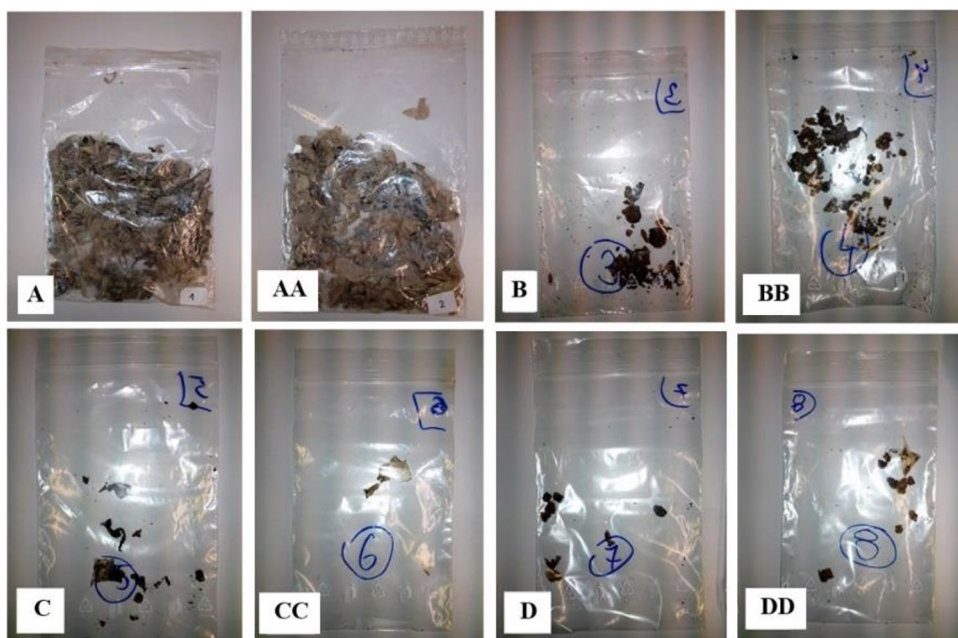
Fig. 4 Photographs of samples once the composting under laboratory conditions ended
