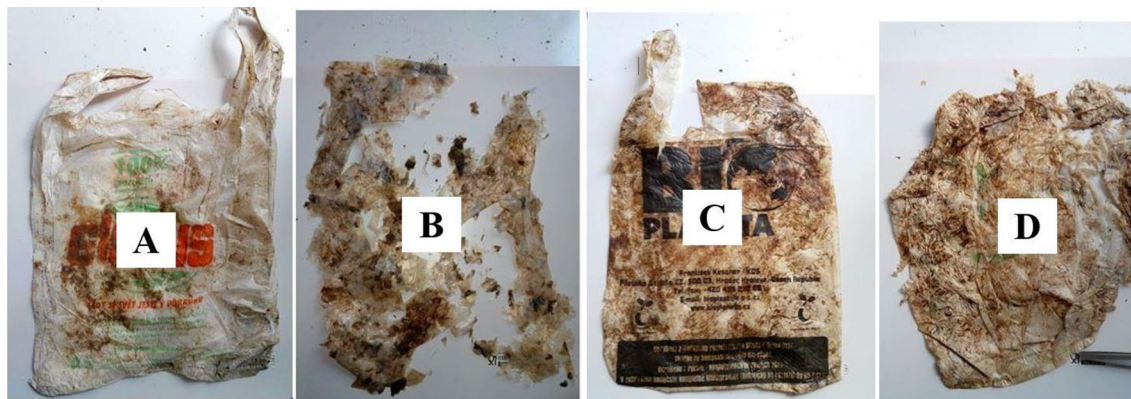
Fig. 7 Photograph of samples after the composting process under real composting conditions was complete
