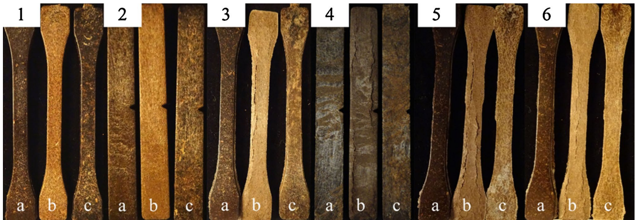
Fig. 6 Composite samples in the form of dumbbells containing 30 wt% (1) or 50 wt% (3) of pine needles, or 50 wt% of mercerized pine needle flour (5) or 50 wt% mercerized pine needle flour with the
