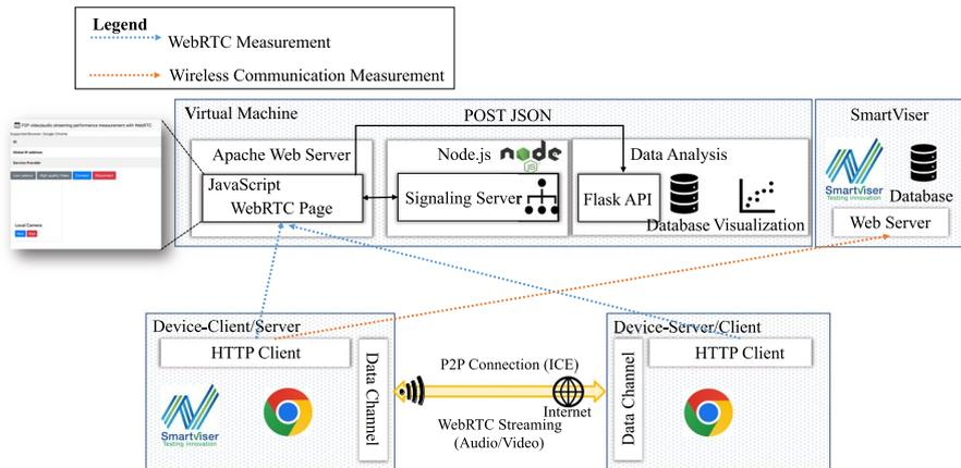
(b) Implementation details of the WebRTC QoS measurement platform
