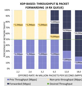
(d) Throughput and packet forwarding in different traffic load scenarios with the ebpf-xdp-based configuration (4 rx-queue).
