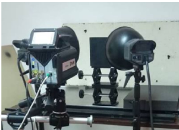
Fig. 5 The used set-up for the thermographic pulsed tests performed on the aluminium specimen
