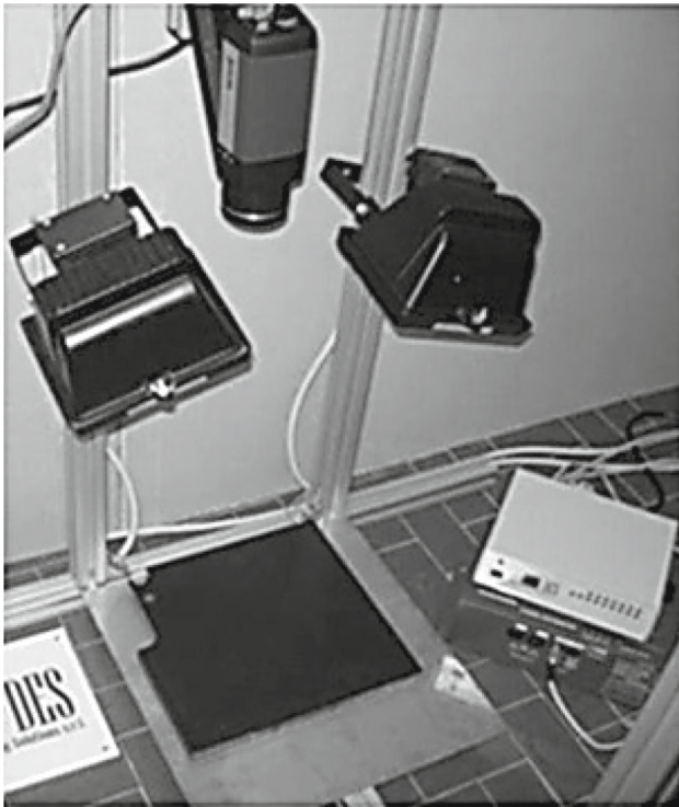
Fig. 7 The used set-up for the thermographic pulsed tests performed on the GFRP specimens [35]
