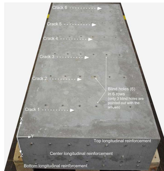
Fig. 1 Photograph of crack specimen after removal of formwork. The blind holes are filled with expansive mortar. Cracks are formed along the dotted arrow directions. The longitudinal reinforcement controls the crack width and depth. The depth of the center reinforcement can be varied by 40 mm up or down to control the crack depth. (The apparent second row of center reinforcement is concrete which filled the blind holes in the formwork which were prepared for the alternate position of the rebars.) (see text for details)
