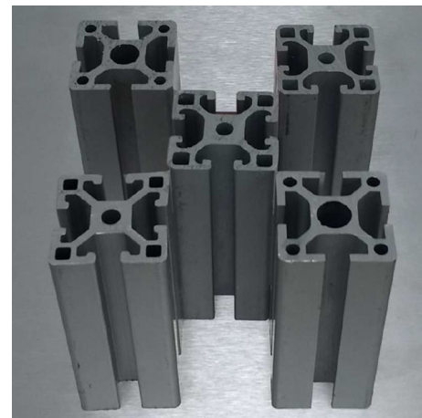
Fig. 3 Aluminum profile measured at our in-house table-top system
