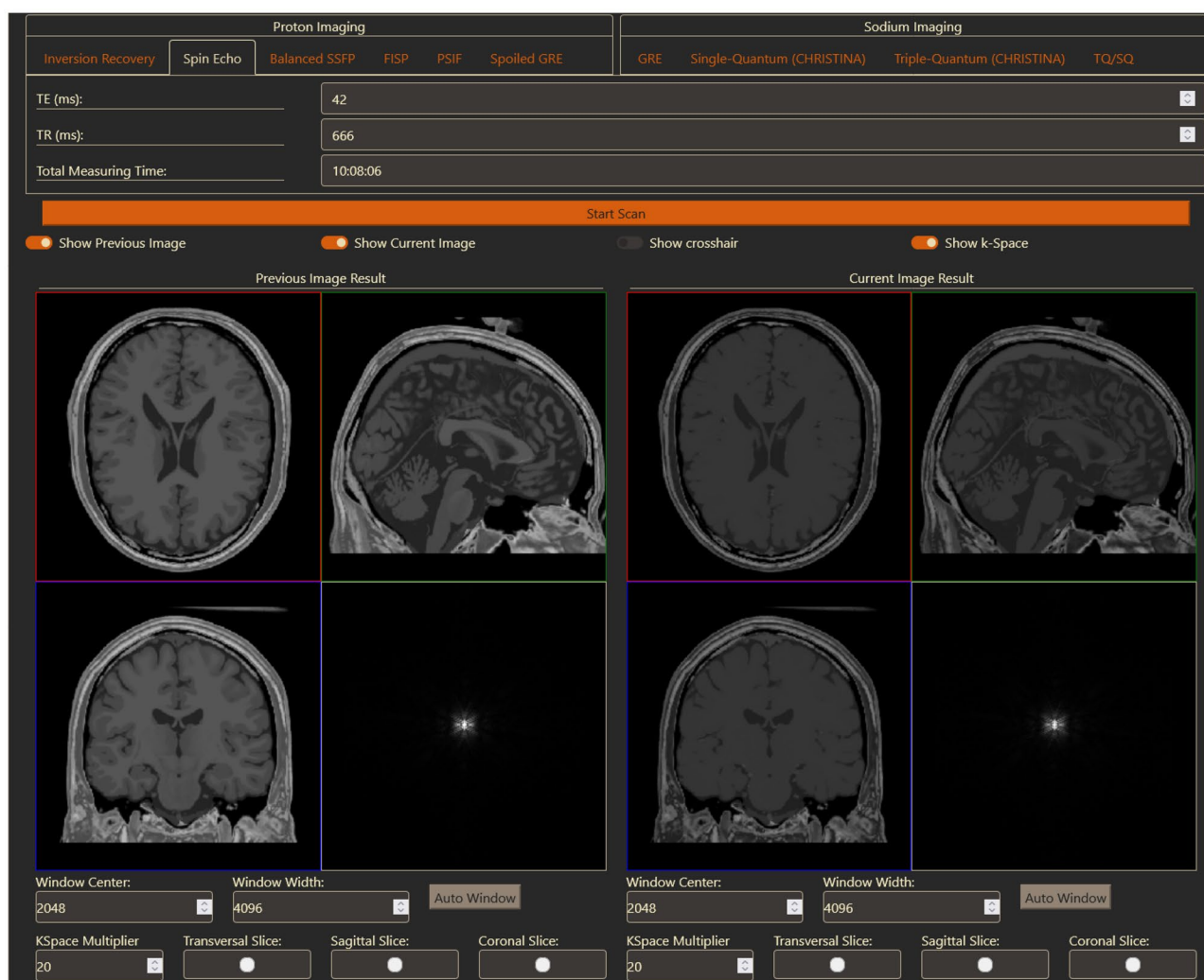
Fig. 4 Generation of a second Spin Echo image. On the left-hand side is the previous Spin Echo image from Fig. 3 and on the right side the new Spin Echo image is shown. The crosshair has been turned off and the 3D view replaced with the k-space
