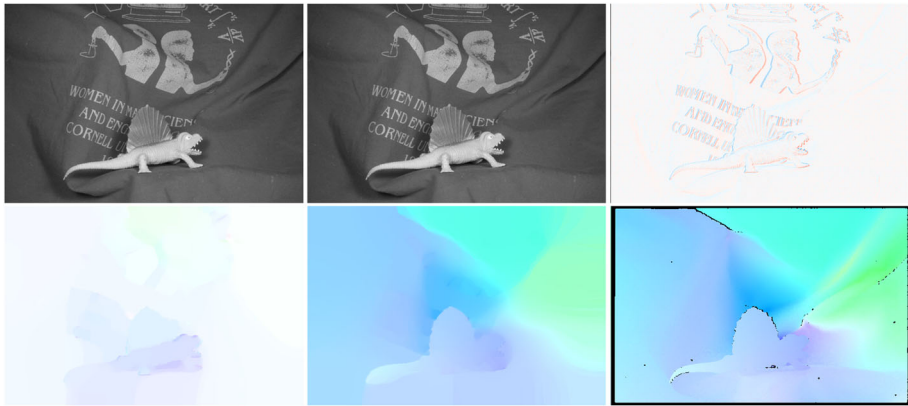
Fig. 7 Middlebury Dimetrodon Optical Flow Benchmark: top row: f_0, f_1 , image difference f_1 - f_0 , bottom left: computed optical flow u using Algorithm 3 stopping after one iteration, bottom center: computed optical flow u using Algorithm 3, bottom right: ground truth optical flow
