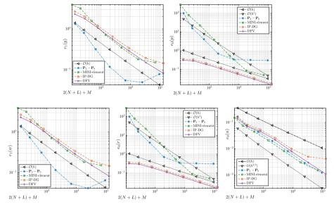
**Fig. 3** Example 1: comparison between errors generated using a  $\mathbb{P}_2 - \mathbb{P}_0$ , the MINI-element, an interior penalty DG, and a DFV approximation of velocity and pressure in the primal and adjoint problems
