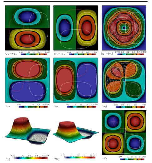
**Fig. 2** Example 1: DFV approximation of state velocity components and magnitude (top panels), components and magnitude of the control variable; approximated with piecewise linear elements (centre row), and state pressure field (bottom row). Contours of the active sets for  $a_1 = a_2$  (in white curves) and  $b_1 = b_2$  (red curves) are displayed (Color figure online)
