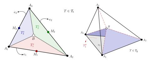
**Fig. 1** Left: sketch of a single primal element T in  $\mathcal{T}_h$ , and sub-elements  $T_i^*$  belonging to the dual partition  $\mathcal{T}_h^*$ . Right: its three-dimensional counterpart, showing a tetrahedron T decomposed into four sub-tetrahedra
