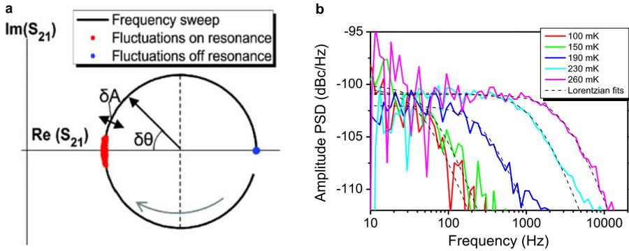
**Fig. 1** (Color online) (a) The real and imaginary parts of the complex transmission  $S_{21}$  as a function of frequency. The *gray arrow* indicates increasing frequency. A resonator amplitude  $A$  and phase  $\theta$  are defined with respect to the resonance circle centre. (b) Power spectral density of the resonator amplitude fluctuations as a function of frequency for six different temperatures, corrected for system noise [4]. The *dashed lines* are Lorentzian fits to the spectra
