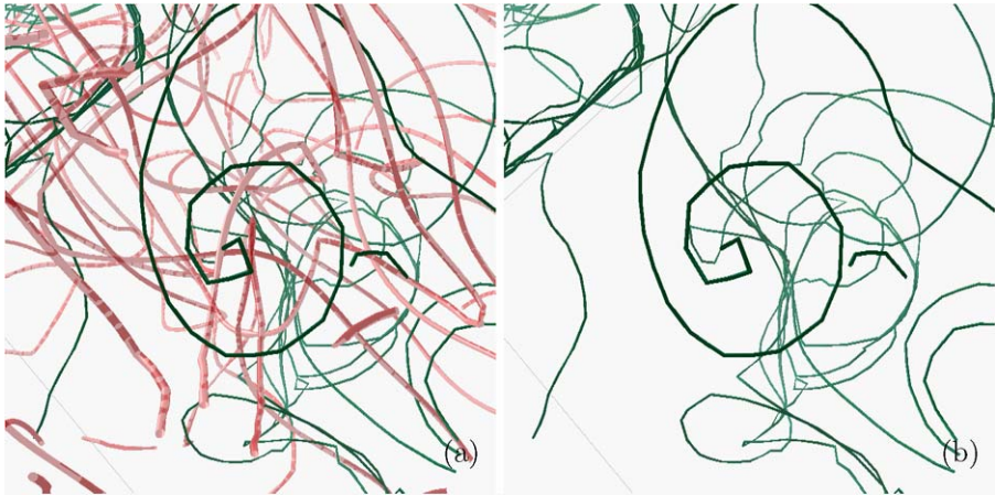
Fig. 5 (Color online) The signature of interaction between intense normal fluid vorticity and quantum vortices in a turbulent velocity field is instability generated spiral-like structures. Left : superfluid vortices together with normal fluid vortices at time t = 1.417 \times 10^{-3} s. For clarity, the vorticity tubes are shown with 0.08 of their actual core radius \sigma . Right : only the superfluid tangle is shown
