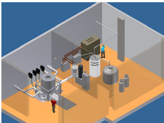
Fig. 1 Schematic drawing of the 45 T hybrid magnet system, that will be constructed in Cell 6 of the HFML, and some of its auxiliary installations
