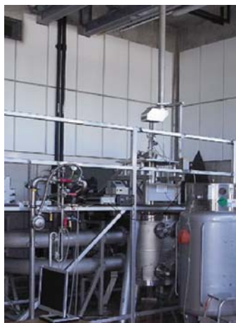
Fig. 3 Left: Coupling of far-infrared radiation from the Bruker interferometer to the sample cryostat using an evacuated beam line assembly; right: far infrared absorption of a cobalt-cluster compound showing the emergence with field and shift of electron spin resonances to 30 T
