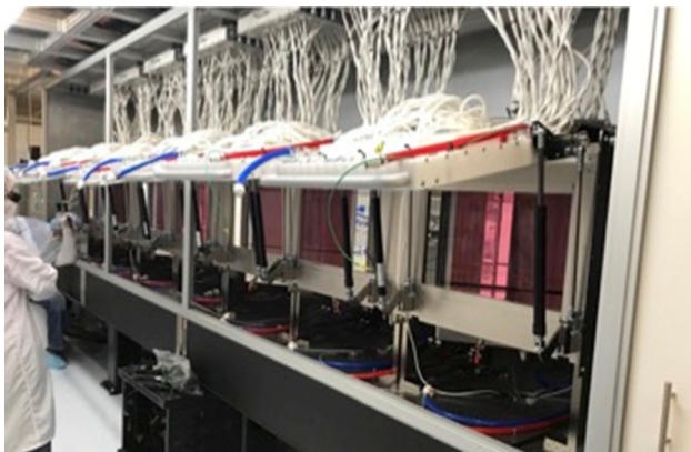
Fig. 17 Photo of liquid cooled 30 cm aperture Nd:glass slab amplifiers used for the ELI-Beamlines L4 ATON laser [78, 79]
