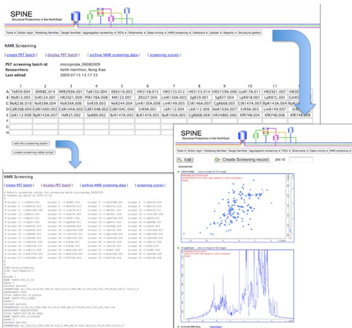
Fig. 5 SPiNE database views showing a “Screening Block” page, push-button generation of IconNMR script for B-ACS 60 sample changer run, and view of the NMR screening record, including 1D and 2D spectra that have been uploaded to the database and made
