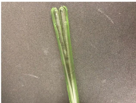
Fig. 8 Cover crack area, with a soft edge
