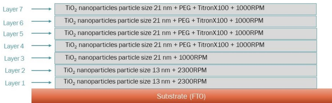
Fig. 1 A schematic diagram to illustrate the configuration of the multilayer photoelectrode with 7 layers of TiO 2 nano-particles
